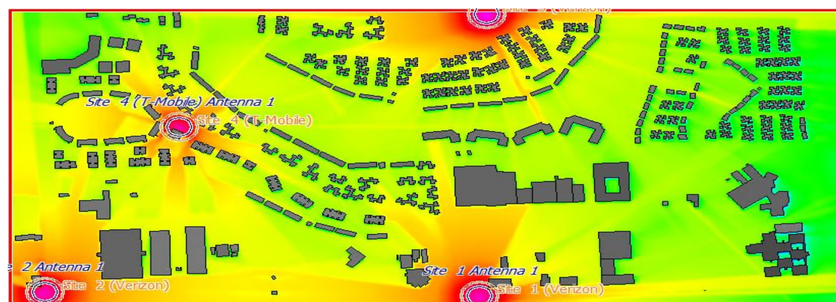
Simulated Coverage Map Made Using Altair WinProp
